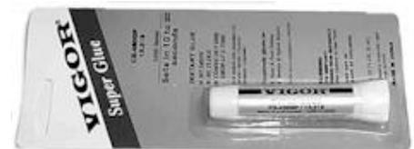
Strong ethyl adhesive bonds any Combination of metal, plastic, rubber, ceramic and glass. Set and cures rapidly at room temperature. Bonds colorless and transparent with almost no shrinkage. 10/20 Series-setting time 10-20 seconds.
